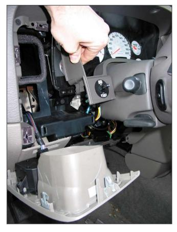
Install the switch into the drilled hole and secure it with the plastic lock ring. Reinstall the dash trim panels by reversing the removal procedure.
