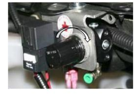
**NOTE**: Over the next two weeks, the backpressure at idle may rise due to initial carbon build up on the inside of the brake housing and on the butterfly. The stop bolt may need to be adjusted again to compensate.
