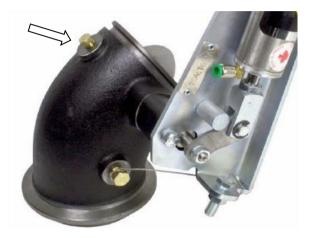
You do not need to measure the air pressure in the system, just the exhaust backpressure, which is located on the cast valve.
