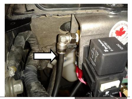
The other line from the compressor is the air suction line. This line is 1/4" diameter and comes with a preinstalled threaded adapter. Install the threaded filter supplied with the air pump into this fitting.
