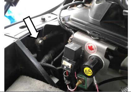
Connect the main power feed to the passenger side positive battery terminal clamp.
